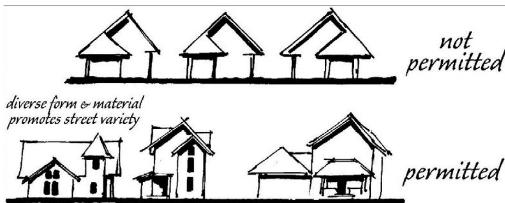
Figure 4-24: Diverse Residential Façades
