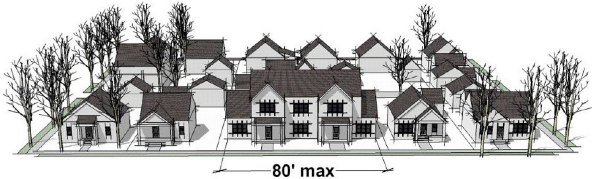
Figure 2-19: Maximum Allowable Length of Multi-Family Residential Structure
